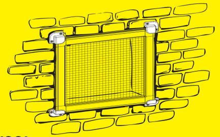
SUPPORTI ANGOLARI IN NYLON PER FISSAGGIO FRONTALE TELAI FISSI
